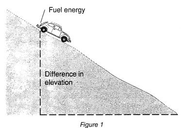
In the same way, to overcome the friction of the moving water against the pipe surface, water flowing along a pipe requires energy. Initially, it is all supplied by the change in altitude (*potential energy*) but it can be converted into an internal energy store known as *pressure energy*.
